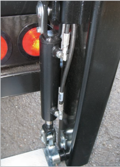
Hydraulic open/close cylinder on the platform
