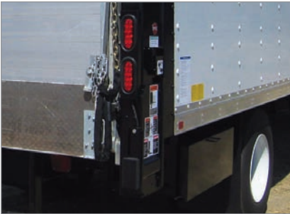
Docking Bumper with recessed backing lights
